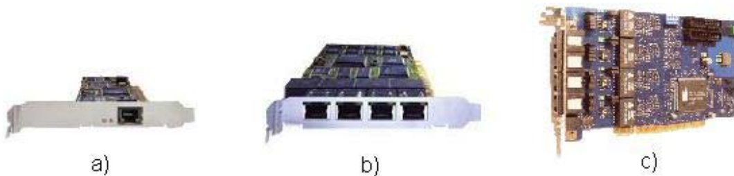
Fig. 2.6 Tarjetas BRI. a) Eicon Networks Diva Server V-BRI , b) Eicon Networks Diva Server 4V-BRI , c) OctoBRI Junghams
